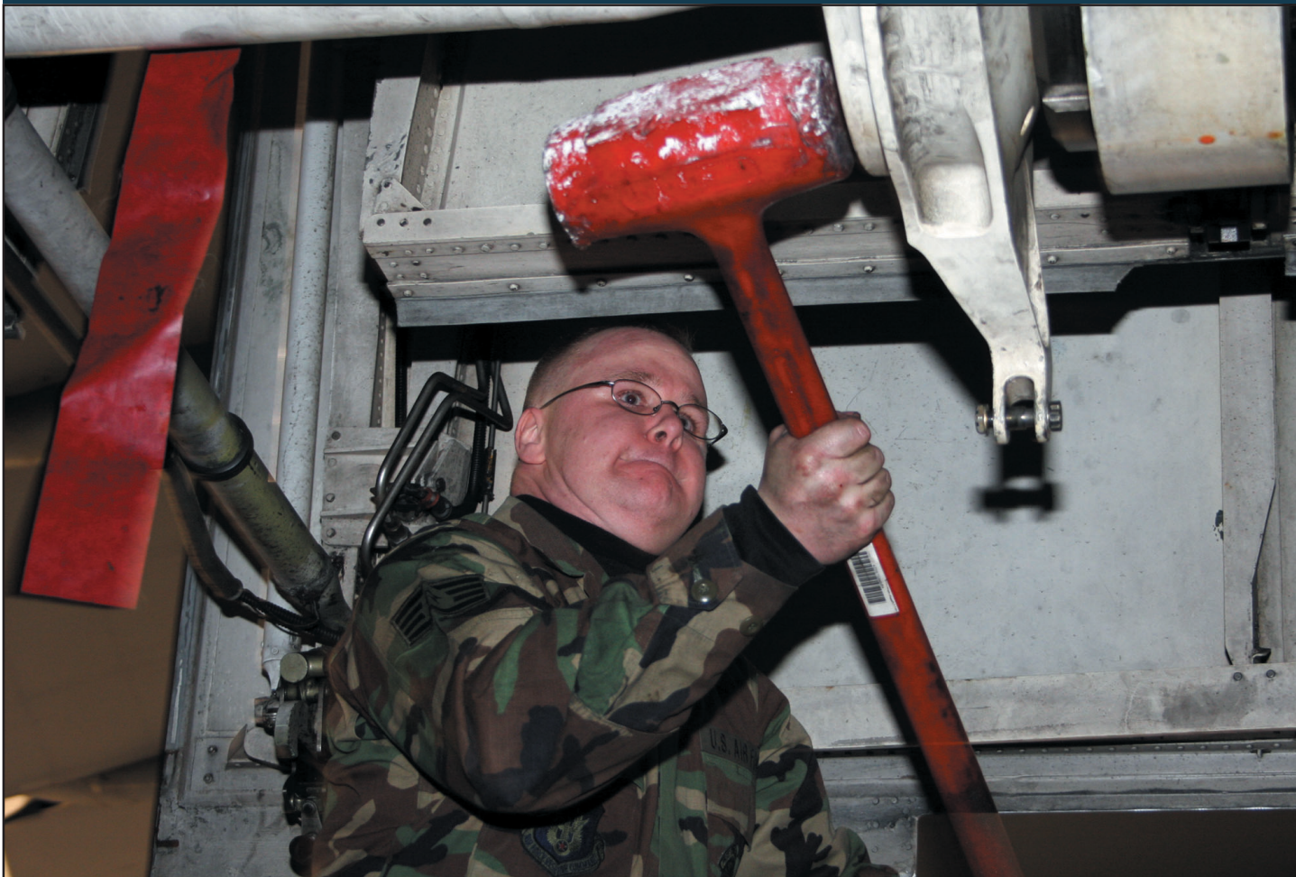
Master Sgt. Stan Evans, 445th Maintenance Squadron, uses all his muscle to get a strut, part of the main landing gear, aligned on a C-5 Galaxy. (Air Force photo/Senior Airman Ken LaRock)
