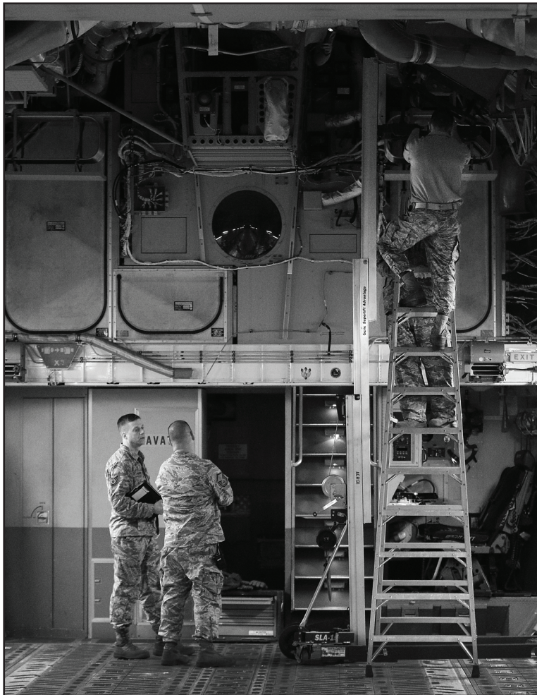
Members of the 445th Aircraft Maintenance Squadron install a life raft inside a C-17 Globemaster III Jan. 8, 2017, during the unit training assembly.
