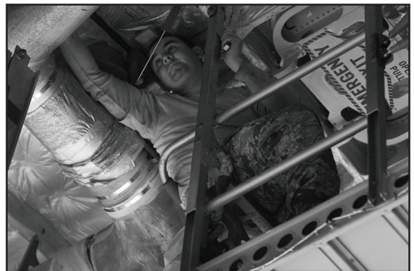
Members of the 445th Aircraft Maintenance Squadron install a life raft inside a C-17 Globemaster III Jan. 8, 2017, during the unit training assembly.
