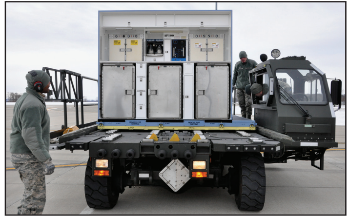
Senior Airman Michael Thompson, left, part of the air transportation crew, secures an air transportable galley-lavatory on a 25K loader for Hickam Air Force Base, Hawaii, in support of exercise Sentry Aloha. Senior Airman Ryan Hood, ramp operations specialist, maneuvers the interior cab controls of the vehicle to operate the mechanized rollers and align the pallet with the steel locking system.
