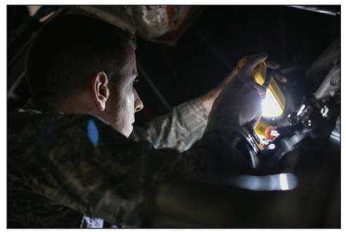
Tech. Sgt. Zachary Stevens, 445th Maintenance Squadron, maintenance technician, inspects a C-17 Globemaster III engine Jan. 6, 2019. The C-17 has four Pratt & Whitney PW2040 (military designation F117-PW-100) engines that produce 40,440 pounds of thrust each.
