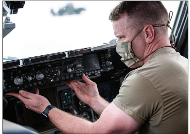
Staff Sgt. Matthew Miklasevich, 445th Aircraft Maintenance Squadron, changes an auto flight control panel of a C-17 Globemaster III, April 13, 2020.
