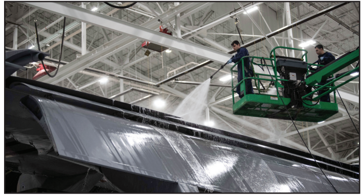
Senior Airman Devin Crider (left) and Staff Sgt. Dominic Fredo, both assigned to the 445th MXG, wash a C-17 Globemaster III, March 27, 2020, to prevent corrosion and ensures lifelong structural integrity of the aircraft.
