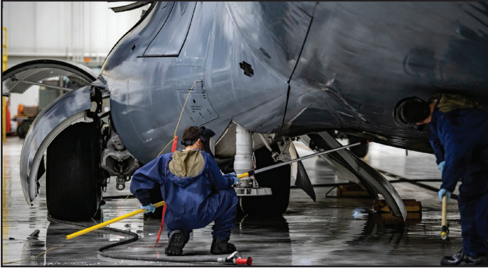
Reserve Citizen Airmen assigned to the 445th Maintenance Group wash a C-17 Globemaster III, March 27, 2020. The wash is part of a process called post aircraft wash corrosion control and is done every 180 days.
