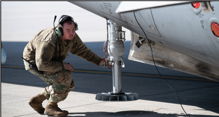
Tech. Sgt. Rodney McElfresh, 445th Aircraft Maintenance Squadron crew chief, verifies strut pressure on a C-17 Globemaster III, April 9, 2020.
